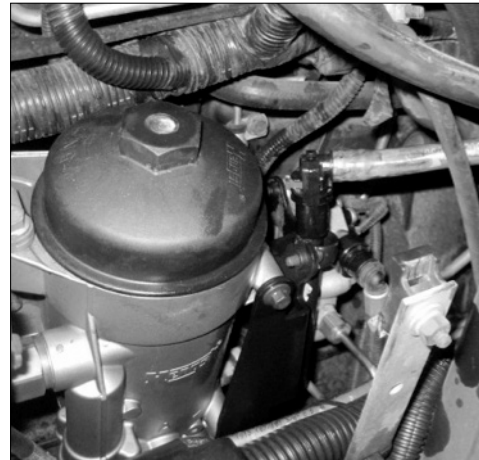
Figure 12: Re-route Return Fuel Line
