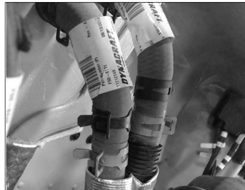
Figure 20: Cab heater circuit
