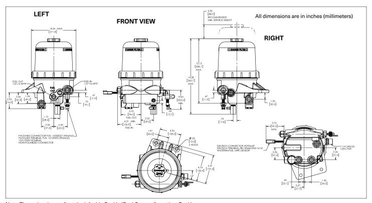
Note: These drawings reflect the left side Fuel In/Fuel Out configuration. Fuel In is also available on the right side.
